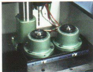
Shuttle Dual 5C Collet Closer Allows operator to load and unload parts while the machine continues to operate. Auto clamp and unclamp of the collet closer. Easy tooling changeover. Simple PLC control package.
