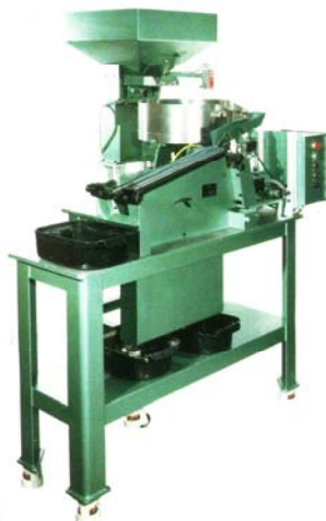
Roll sorters are used for sorting parts by head diameter or washers and nuts by thickness.
