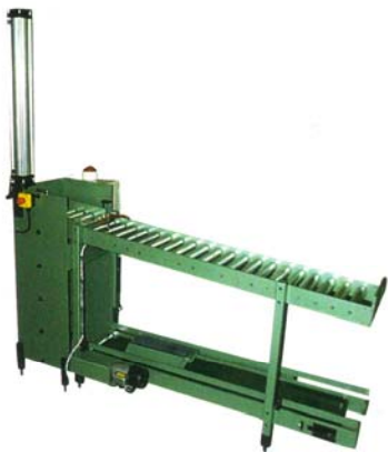
Packaging conveyors facilitate the flow of parts away from the machine at a higher level and in a more controlled way.
