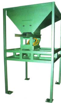
12 cubic foot storage hopper for automatic loading of the feeder bowl. Supplied with high level sensor to turn the hopper on and off when needed.
